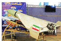
IRAN System: Shahed-136 (swarms) Type: Loitering munition Swarm Size: 10-50 Range: 2,000 km Features: GPS-guided, low radar signature, low-cost
