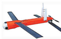
USA System: LOCUST Type: Micro UAV swarm Swarm Size: 50-100 Range: 30-60 km Features: AI coordination, launched from tubes
