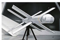
RUSSIA System: Lancet & Shahed Type: Loitering + fixed-wing Swarm Size: 5-20 Range: 40-300 km Features: Used in layered attacks with multiple decoys
